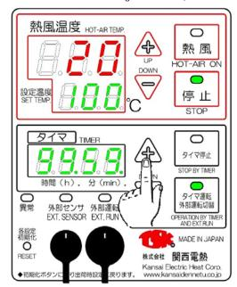
③ Press the hot air switch. The dot on the timer flashes and the countdown starts.
