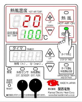
After use, turn off the power switch and turn off the factory power supply (primary power supply). Immediately after use, there is residual heat in the main body and discharge port, so make sure that it has cooled sufficiently before storing it.
