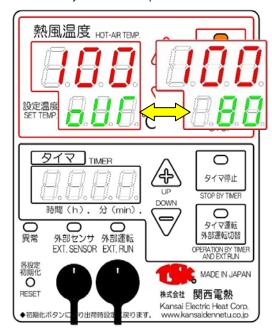
※ Press the hot air switch again to end the output display.
