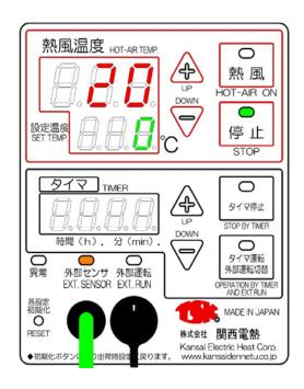
3 Set the temperature of the place controlled by the external sensor.
