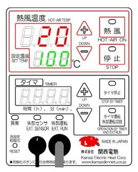
3 Timer operation Press and hold the external operation selector switch (5 seconds or longer).
