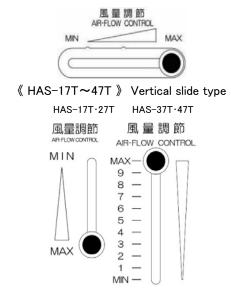
If the air volume is large, the set temperature may not be reached to the temp you require, so refer to the performance curve described in the catalog and use only the appropriate air volume.
