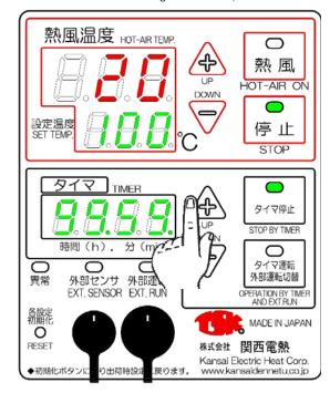
3 Press the hot air switch. Hot air operation is started, and at the same time, the dot on the timer flashes and the countdown starts.
