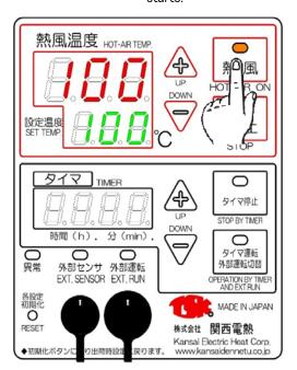
② Use the up and down keys to set any hot air temperature.
