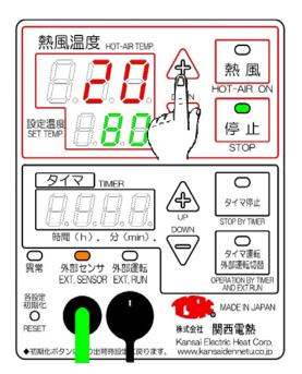
When the hot air switch is pressed, the hot air lamp (orange) lights up and hot air operation starts at the set temperature of the external sensor.
