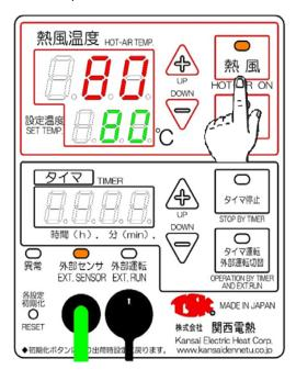
If the external sensor is removed during operation, the abnormal lamp (red) lights up and the external burnout is abnormal (hot air temperature display:
