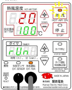
With the operation on / off 1-COM turned on, turn on the heater on / off 4-COM. Start hot air operation.
