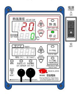
When you press the hot air switch, the hot air lamp (orange) lights up and hot air operation starts.
