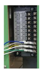
XAfter connecting, be sure to reattach the service terminal cover, and fix the remote cable to prevent the terminal part from being pulled.
