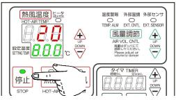
If you do not use the super heater for a long time, turn off the power supply on the factory side.
