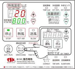
The factory lock mode is "Lc1". "---" unlocks, "Lc2" locks only temperature setting, air volume setting, timer setting, and other settings. If you want to fix the temperature setting, air volume setting, and timer setting and prevent erroneous setting, you can change it to "Lc2" and use it.
