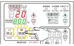
The hot air lamp (orange) lights up and hot air operation starts.
