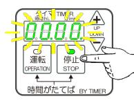
② Use the up and down keys to set time.you desire It can be set in 1 minute increments up to 99 hours 59 minutes. When you release the up / down key after completing the setting, the setting value will be registered by switching from blinking to lit after 2 seconds.
