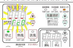
The display of each sensor blinks in the hot air temperature section and in the set temperature section.
