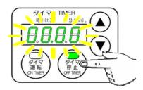
*Please set up it to optional time by the up down key. Timer can be set up until 99 hours 59 minutes. After setting, please separate the hand from the up down key. Flickering changes to illumination 2 seconds later and setting value is registered.*
