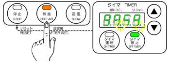
Time counting (Reduction of timer setting) is started (Dot display flickering) and hot-air operation is started. Hot-air operation is stopped when the time counting becomes 00.00. HOT-AIR lamp (Orange) is lighted during hot-air operation, and is changed to flickering after the hot-air operation completion.
