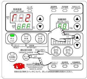
*③Please set up optional cooling time by the up* down key. After setting, please return to the display of usually operation condition by pushing the MODE switch 1 time.
