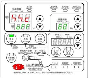
*Please start hot-air operation.* EXT. CNTL lamp (Orange) is lighted irrespective of the input of the external temp. control in the case that external temp. control setting was changed to ON.
