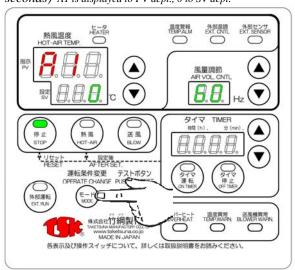
*③Please change OFF of SV dept. to ON by the up key.* After setting, please return to the display of usually operation condition by pushing the MODE switch 1 time.
