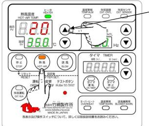
Setting of hot-air temp. It can change in 0 to 350 °C range by the up down key. \* Max. setting temp. of TSK-51HT is 500 °C.
