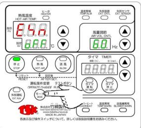
Please start hot-air operation. EXT. SENSOR lamp (Orange) is lighted in the case that external sensor setting was changed to ON.
