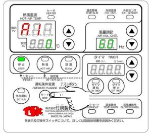
XOperation of this machine is not stopped by the temp. alarm.XTemp. alarm output is ineffective when setting of temp. alarm is 0.
