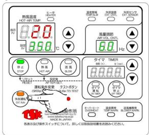
**2**Please operate by the external operation signal. BLOW lamp (Green) is lighted and this becomes blow operation when external operation signal is ON and enternal heater ON/OFF signal is OFF.
