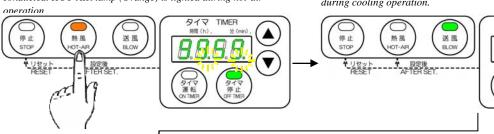
Cooling operation is stopped when time counting became 00.00. And, Blow lamp is flickered.
