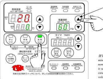
Setting of air volume control (Setting of the frequency) It can change in 30Hz to 60Hz range by the up down key.
