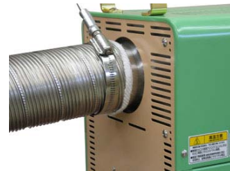
Execution example of the glass tape for the air leakage prevention
