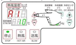
(3) Please start hot-air operation. Alarm is output from the service terminal and TEMP.ALM lamp (Red) is lighted when hot-air temp. becomes more than +10 °C or less than -10 °C if "10" were set up. (Excerpt for temp. rising at the time of the hot-air operation start.)
