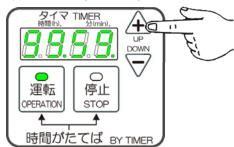
Time counting (Reduction of the setting time) is started (Flickering of the dot display), and hot-air operation is started when the time counting becomes to "00.00.". And, HOT-AIR lamp (Orange) is flickered during time counting, and the lamp changes to lighting after hot-air operation was started.
