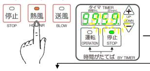
Cooling operation (Blow operation) is stopped when the time counting becomes to "00.00.", and BLOW lamp (Green) is flickered.
