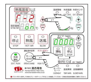
**4** Please set up the hot-air operation time by pushing STOP BY TIMER.
