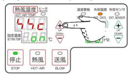
(5) Please start hot-air operation after setting the optional temp. and air volume, and please start even temp. control by the temp. controller of the outside simultaneously.
