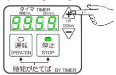
Time counting (Reduction of the setting time) is started (Flickering of the dot display), and hot-air operation is started. Hot-air operation is stopped when the time counting becomes to "00.00.". And, HOT-AIR lamp (Orange) is lighted during hot-air operation, and the lamp changes to flickering after hotair operation was started.
