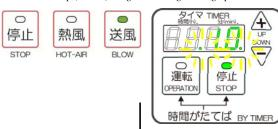
\* Timer operation is stopped by pushing STOP switch. (Timer setting is returned to the initial setting value.)
